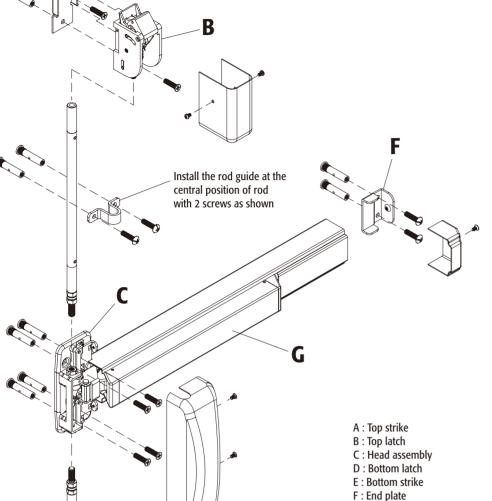
Install the rod guide at the central position of rod with 2 screws as shown
