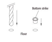
Step 1: Drill ø 25/32" (20mm), depth 25/32" (20mm) on floor.
