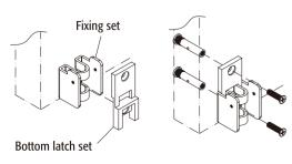
Step1: Attach the bottom latch set to the fixing set. Step2:
